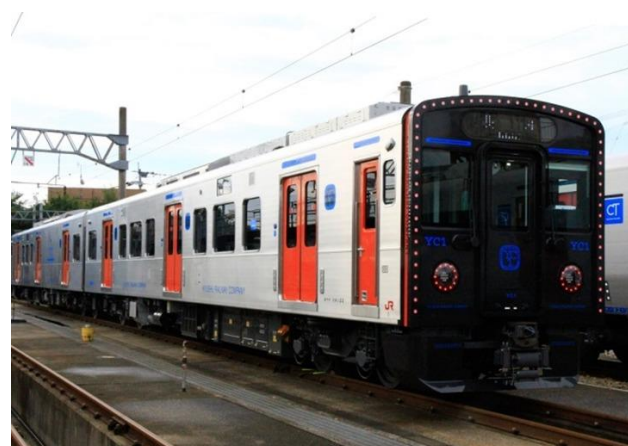
YC1 series diesel-electric rolling stock equipped with storage battery
