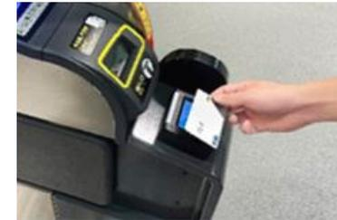
We became the first company in the JR Group to introduce, on a trial basis, a service that allows passengers to use trains by passing a Visa touch payment-compatible card or smartphone over a dedicated terminal at an automatic ticket gate.
