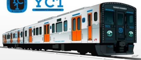
【YC1 series storage battery-equipped diesel-electric (hybrid) rolling stock】
