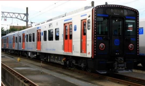
YC1 series diesel-electric rolling stock equipped with storage battery
